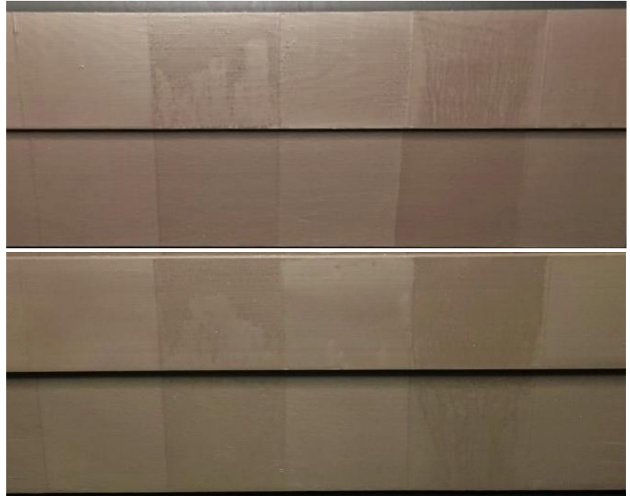
Comparison of Accelerated (top) and Exterior Exposures (bottom)
