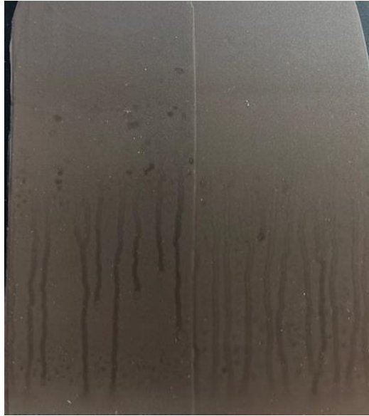
Cleveland Condensing Test (ASTM 4585)
