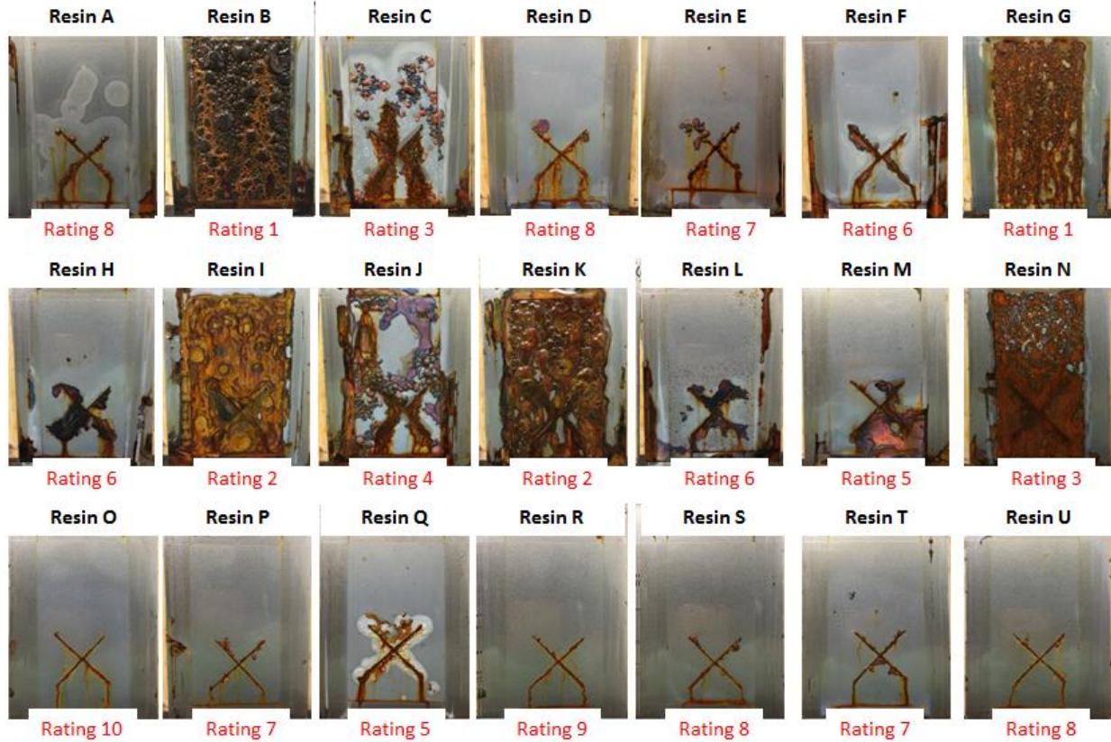
Figure 8: Corrosion results (560hrs B117) and ratings of Resin A through U (3-3.5mil DFT, CRS).
