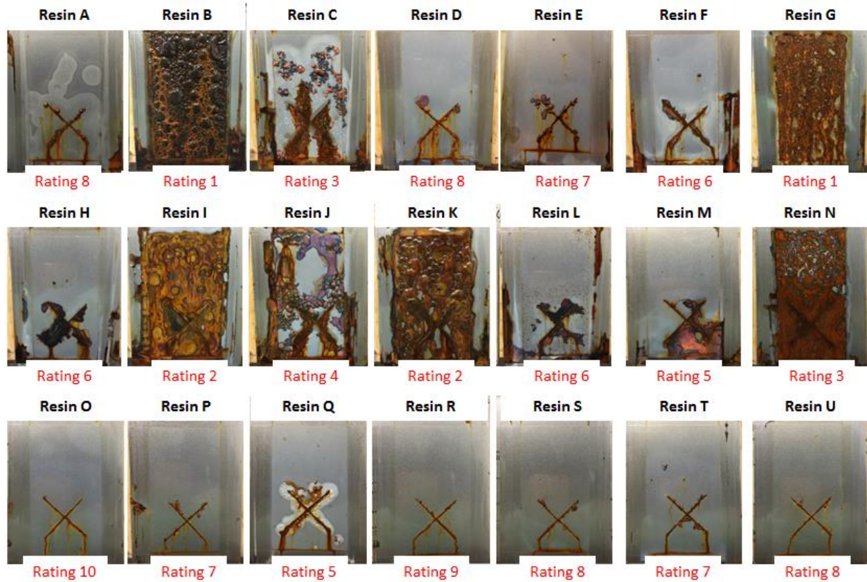
Figure 9: Corrosion results (560hrs B117) and ratings of Resin A through U (3-3.5mil DFT, CRS)
