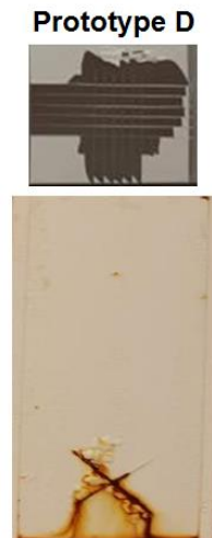
Figure 3: Aluminum adhesion vs. corrosion resistance on CRS (2mil DFT, 400hrs B117) of Prototype D
