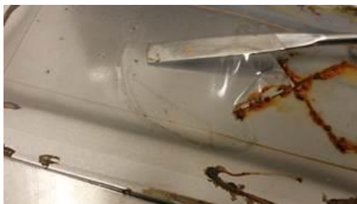
Figure 8: Loss of adhesion after 300hrs exposure to the B117 salt fog cabinet
