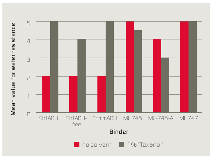
Figure 3: No-VOC coalescent influence on polymer water resistance.
