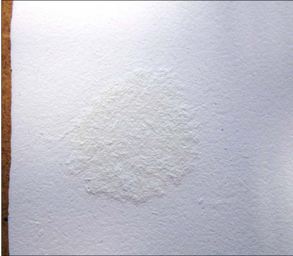
Water resistance (1h) of basecoat, spray applied - 120 g/m 2 , 1 week at RT
