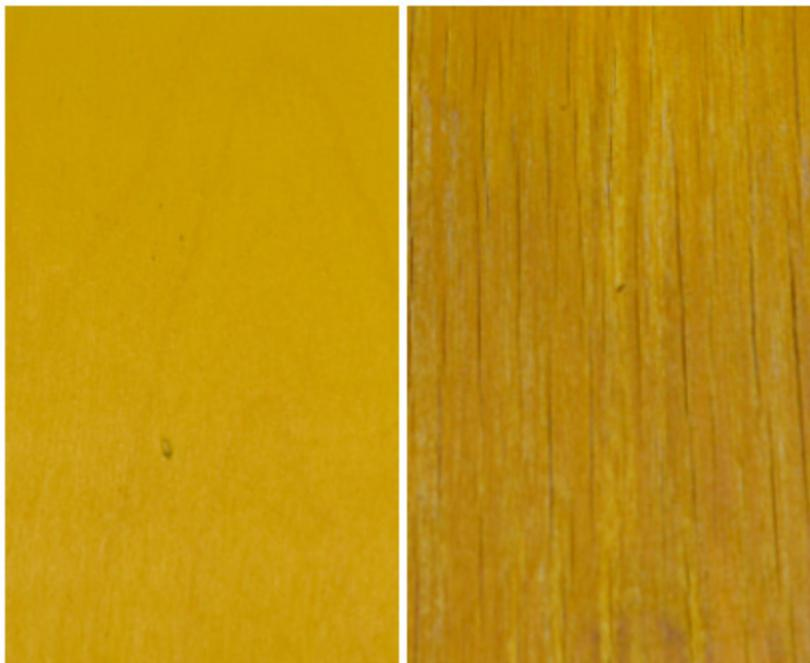
Figure 15: NovoColor® SF 8113 organic yellow unexposed (left) compared to 2000-hour QUV® exposure (right)
