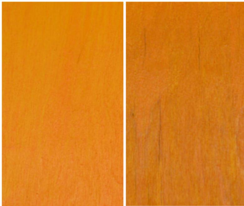
Figure 17: NovoColor® SF 8115 golden yellow unexposed (left) compared to 2000-hour QUV® exposure (right)
