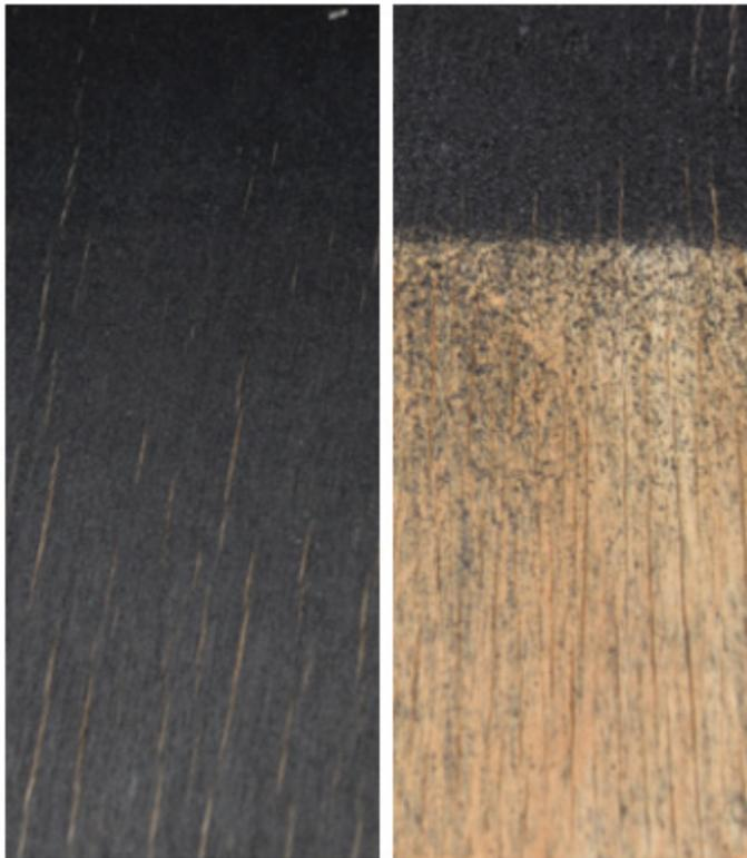
Figure 20: 2000-hour QUV® exposure black (left) compared to colored dye (right)
