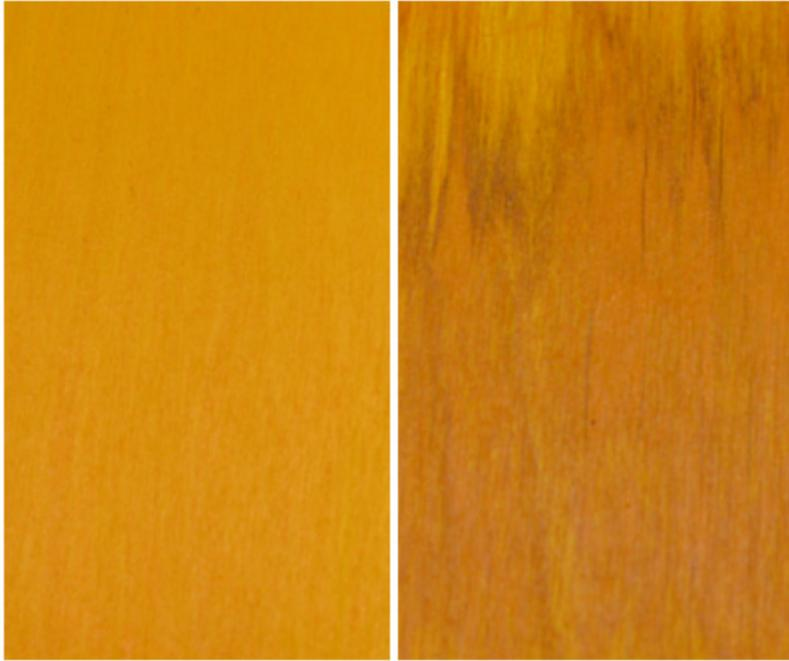
Figure 16: NovoColor® SF 8114 medium yellow unexposed (left) compared to 2000-hour QUV® exposure (right)
