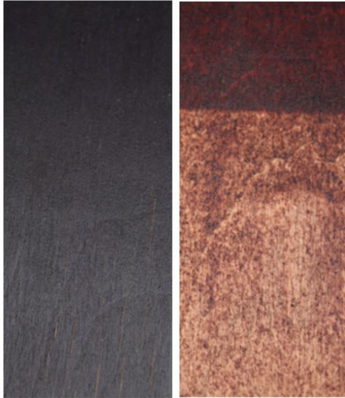
Figure 19: 2000-hour QUV® exposure brown (left) compared to colored dye (right)
