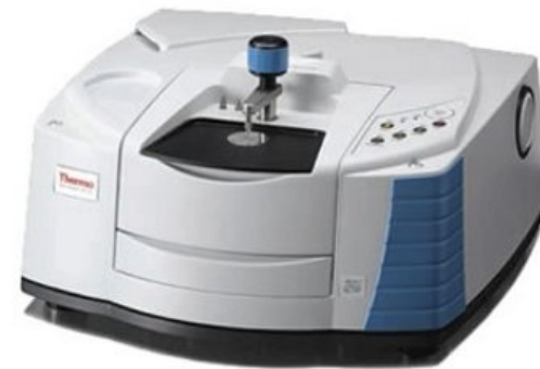
Thermo Fischer Nicolet iS10 with Smart iTR fixture
