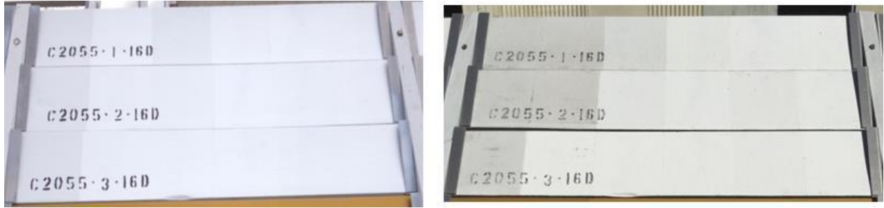
Figure 4: Semi-gloss benchmark series – initial and 7 month Los Angeles exposure.
