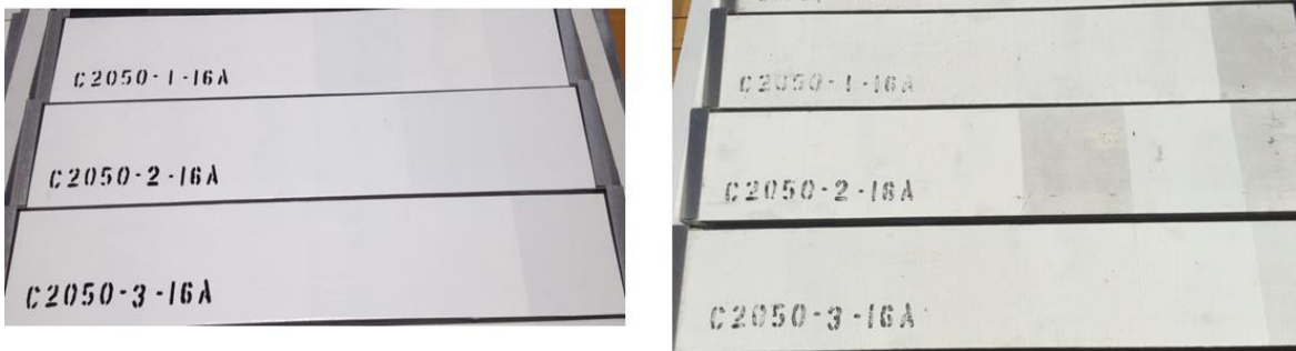
Figure 3: High gloss benchmark Series – Initial and 10 month Los Angeles exposure.
