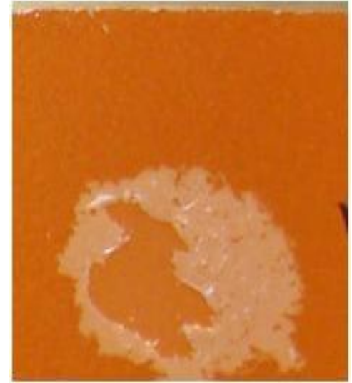
De-bonding due to chemical exposure
