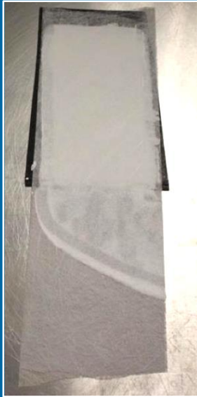
Coating Applied with Fabric Embedded
