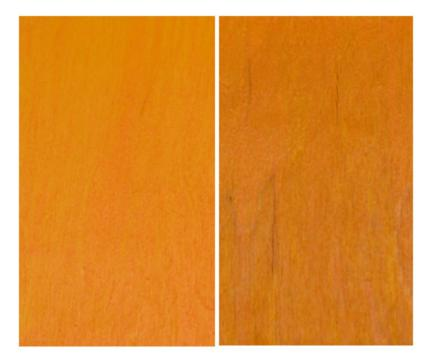
Figure 17: NovoColor<sup>®</sup> SF 8115 golden yellow unexposed (left) compared to 2000-hour QUV<sup>®</sup> exposure (right)
