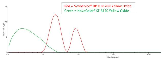
Figure 14: Particle size distribution of yellow iron oxide colorants
