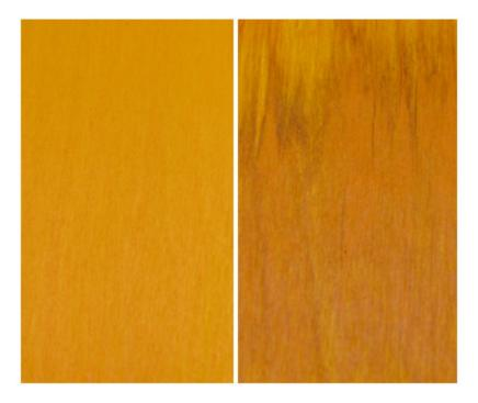
Figure 16: NovoColor<sup>®</sup> SF 8114 medium yellow unexposed (left) compared to 2000-hour QUV<sup>®</sup> exposure (right)
