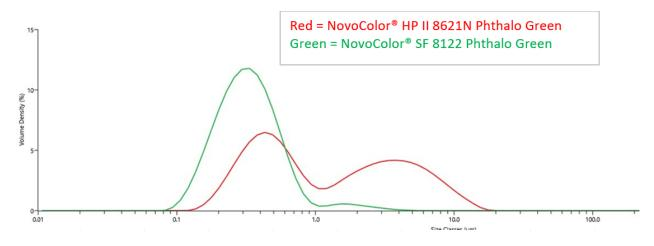
Figure 11: Particle size distribution of phthalo green colorants
