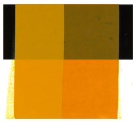
Figure 7: Transparency of yellow iron oxide colorants. NovoColor® HP II (left) NovoColor® SF (right)
