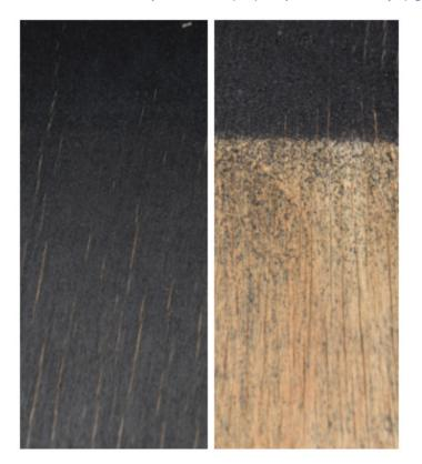
Figure 20: 2000-hour QUV<sup>®</sup> exposure black (left) compared to colored dye (right)
