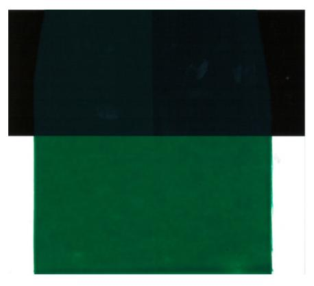
Figure 4: Transparency of phthalo green colorants. NovoColor® HP II (left) NovoColor® SF (right)
