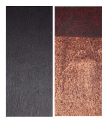
Figure 19: 2000-hour QUV® exposure brown (left) compared to colored dye (right)
